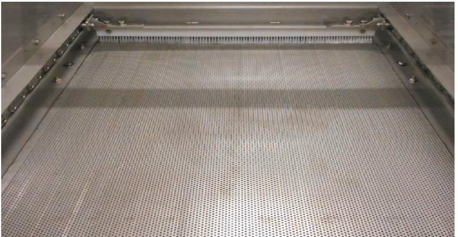
Perforated plate with brushes on a CPS screen
