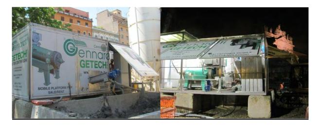
3) 40' container, whose centrifuge has a 75 kW motor and its mud capacity is 20 – 50 cubic meters per hours, depending on the physical – chemical characteristic of the sludge, 12 tph of dry solids.
