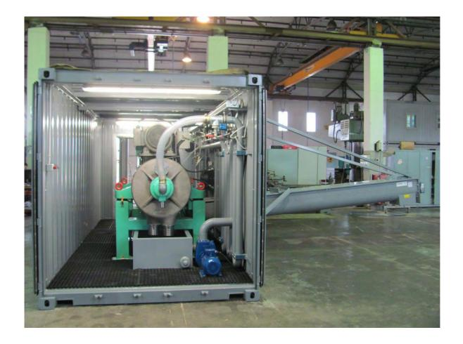
Our business continues to be the design and the construction of centrifuge decanters and their containerized turn key plants (liftable on a truck/ship).
