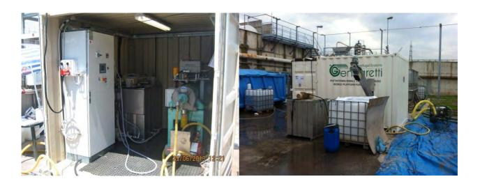
2) 6,2 m. x 2,2 m., height 2,7 m., mobile plant, whose centrifuge has a 30 kW motor and its mud capacity is 8 – 15 cubic meters per hours, depending on the physical – chemical characteristic of the sludge, 3 tph of dry solids.
