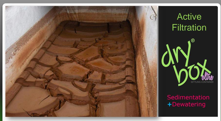
Result of mud dehydration shown 36 hours after activation of the dynamic filter.
