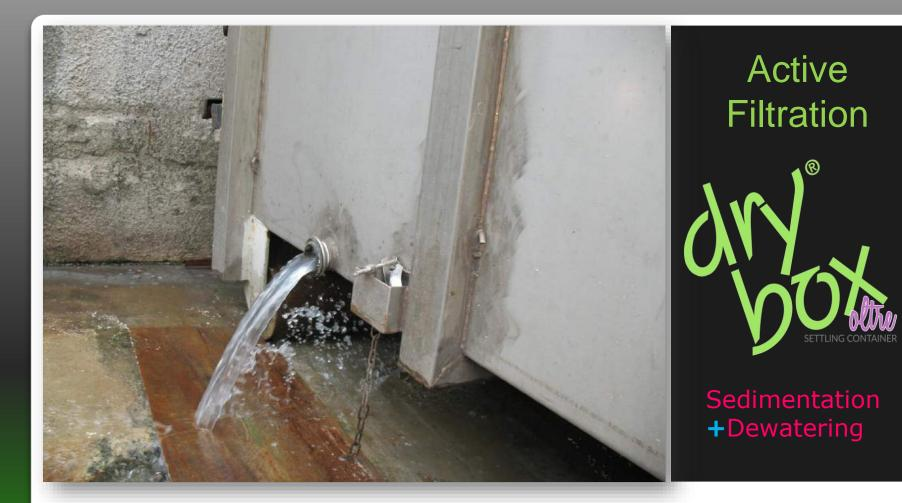
Discharge of filtered water with collecting pit, quick nozzle and door box
